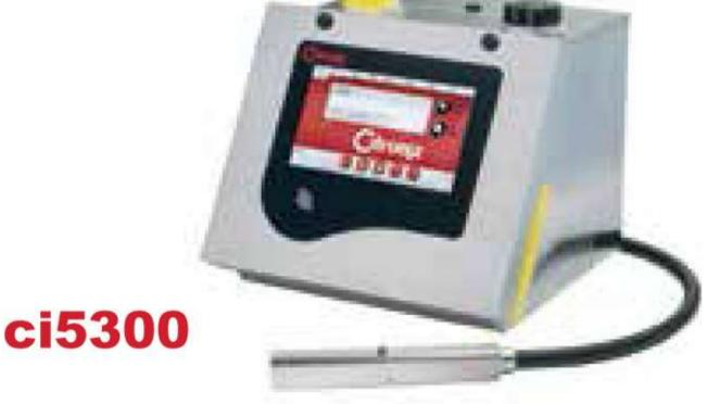
Intermediate printer in stainless steel cabinet to meet 1 to 3 line printing applications with Macro and Normal drop size at speeds of up to 9.8m/s. Designed for all non-pigment ink types.
